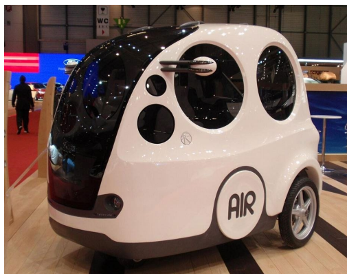
Fig. 1. This car runs on a pneumatic engine (Photo taken from the official website of Motor Development International)
